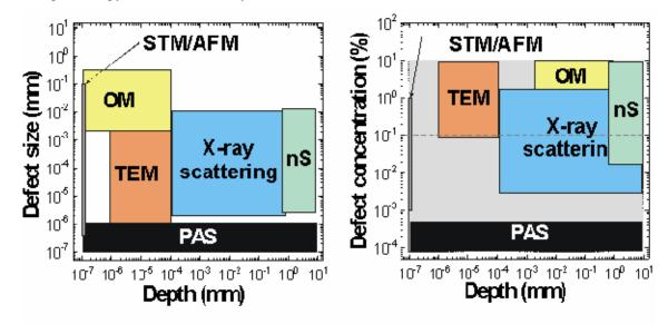
Fig. 5. General overview of applicability range for some spectroscopy techniques.
